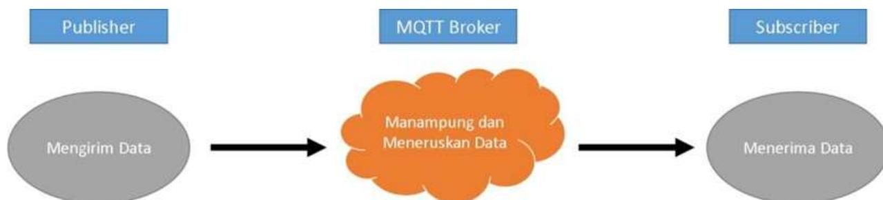
Gambar 5. Alur sistem MQTT *Broker*
